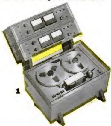
A SEEMING IMPOSSIBILITY —playing four channels from a single record groove—is accomplished by this Japanese Victor decoder to be marketed soon. It will work with any high-frequency phono pickup
